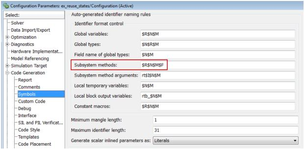
This enhancement enables you to control the format of generated function names for atomic subcharts when building an embedded real-time (ERT) target. For more information, see Generating Reusable Code for Unit Testing in the Stateflow User's Guide.
