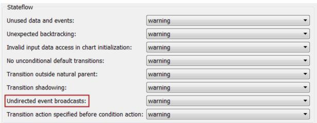
Undirected local event broadcasts can cause unwanted recursive behavior in a chart and inefficient code generation. You can avoid this behavior by using the send operator to create *directed* local event broadcasts. For more information, see Guidelines for Avoiding Unwanted Recursion in a Chart and Broadcasting Events to Synchronize States in the Stateflow documentation.
